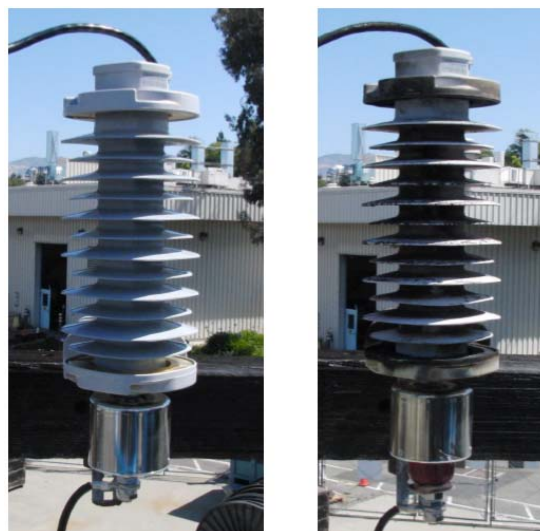
Figure 9 Testing of Siemens 24 kV Arrester
