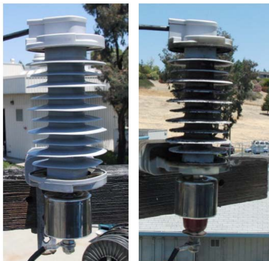
Figure 8 Testing of Siemens 15 kV Arrester
